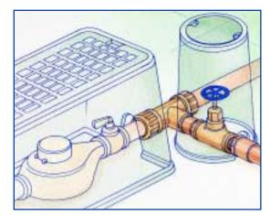
P.O.C. Non-Freezing: Use a brass compression tee to connect your sprinkler system to the household water supply.
