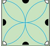
**Step 1** Corners are critical points. Start by placing sprinklers in each corner.
