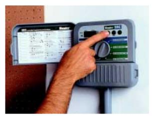
An automatic controller stores information on what days to water, what time to start watering and how long each zone will run.
