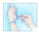
Assembling PVC: 1. Place solvent on inside of fitting and outside of pipe.
